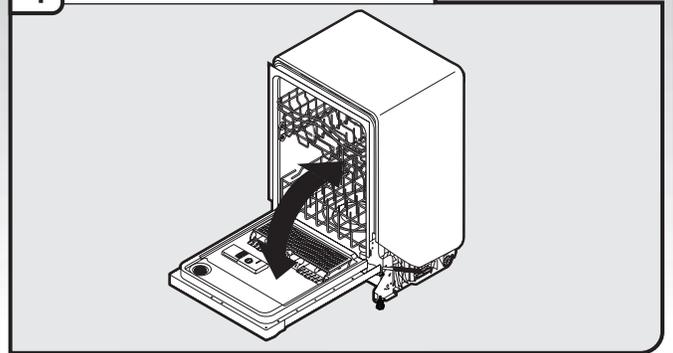
With another person holding the dishwasher to keep it from tipping, open and close the door a few times. If the door closes or falls open under its own weight, the door tension will need to be adjusted.
